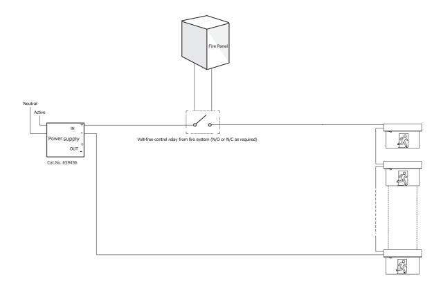
Note: Max. cable length over entire loop when using shielded twisted pair cable is 500 m.
